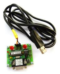
The simulator is put into serial comms mode by setting its PF or TF switch (or both) to **position '1'**. The simulator then listens to commands at **1200Baud**, 1 start-bit, 8 data-bits, 1 stop-bit. Commands are all ASCII, so any terminal software can be used.
